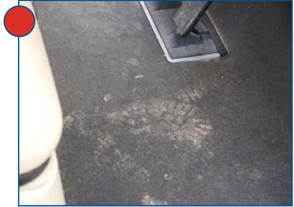
Floor mat unacceptable
